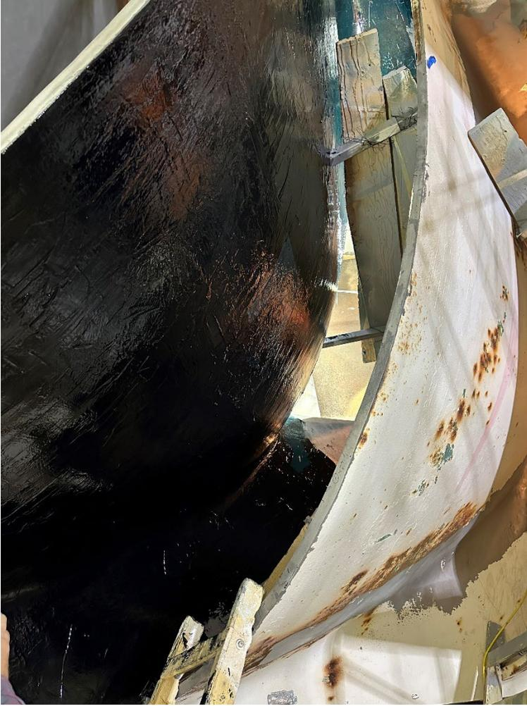
Figure 6.—Blade 13 shown coated with PE1.
