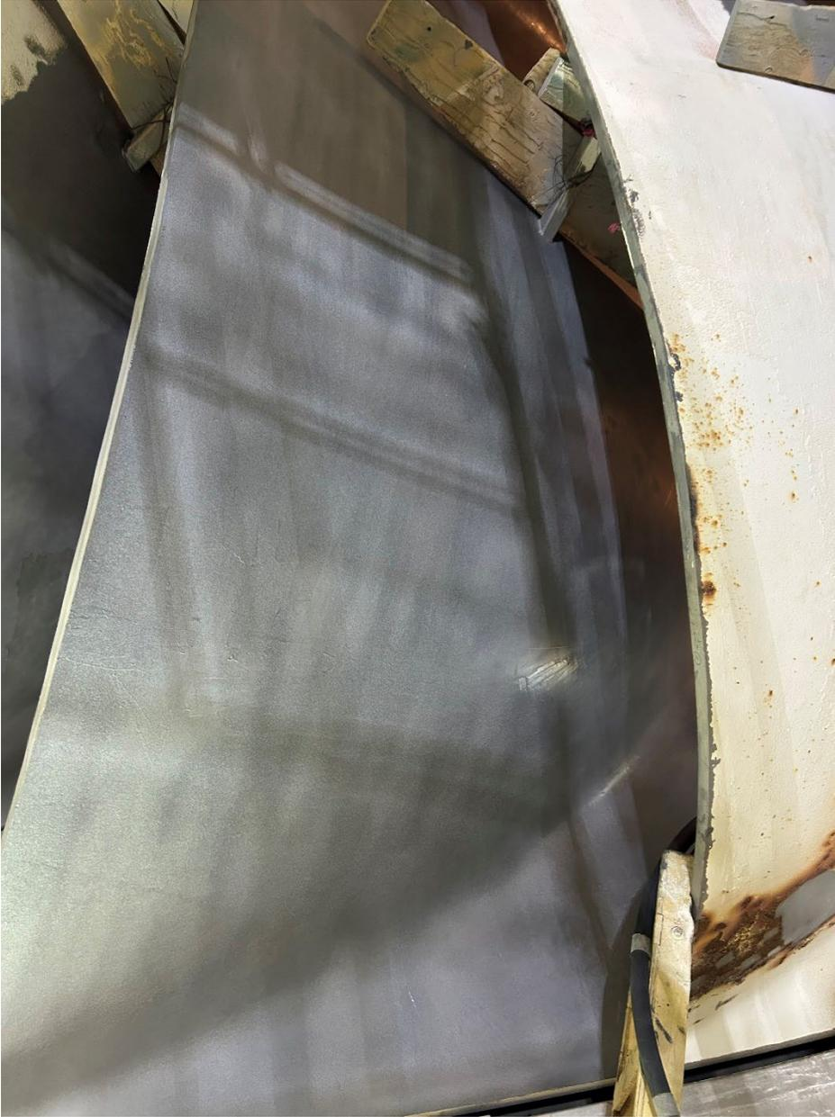
Figure 2.—The surface of Blade 13 primed with ceramic-filled epoxy, shown after sweep blasting.
