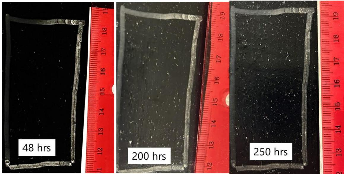
Figure 23.—PE 2-1 long-term cavitation, notice the damage is not visible. Ruler is in millimeters.
