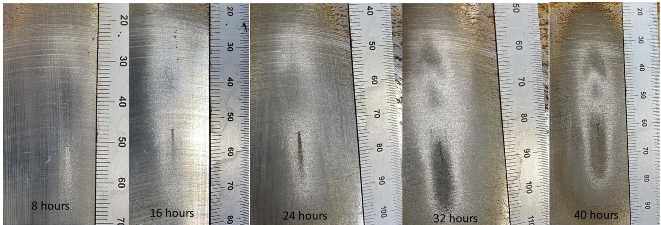
**Figure 5: Baseline testing of mild steel and progression of cavitation damage.**
