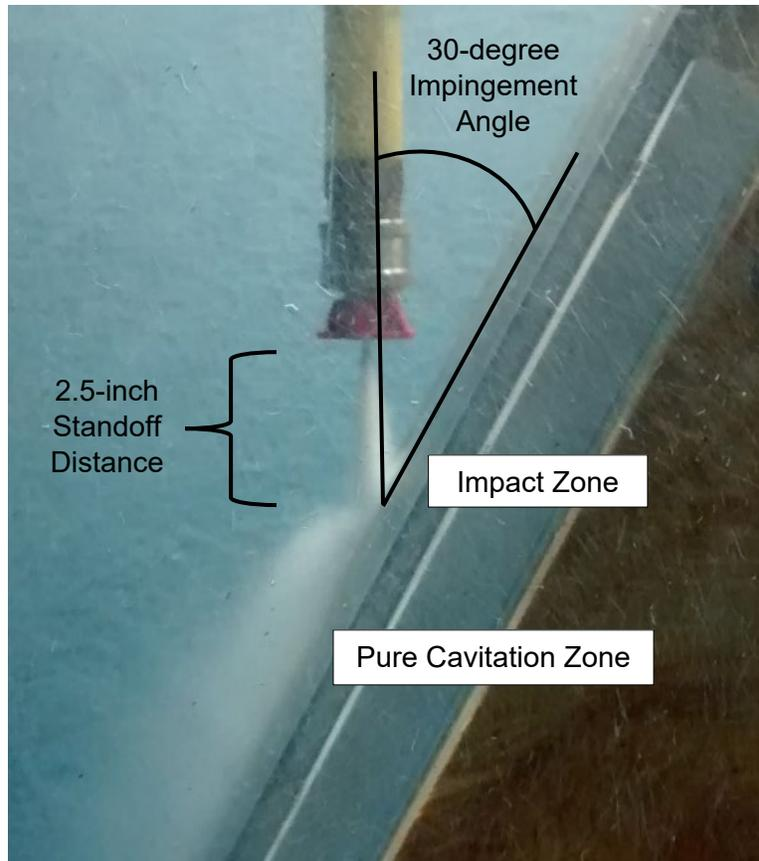
**Figure 2: Submerged jet cavitation showing the sample angle with the cavitation travelling down the sample, along with the location of the two defining zones of damage.**
