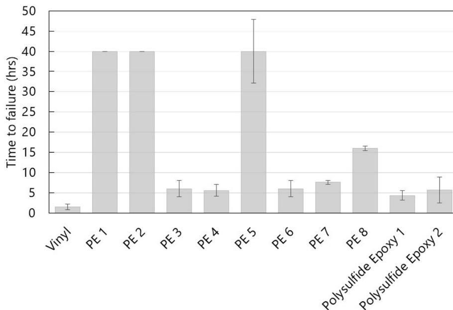
Figure 12.—Cavitation resistance of elastomeric coatings from laboratory testing with time to failure in hours (hrs).
