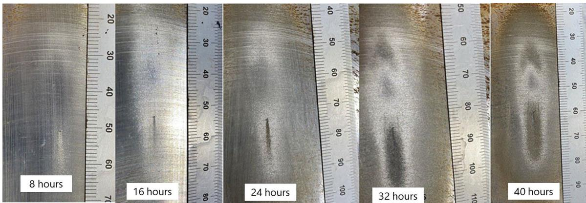
Figure 10.—Baseline testing of mild steel and progression of cavitation damage after increasing 8-hour test periods, shown from left to right. Ruler tick marks are in millimeters.
