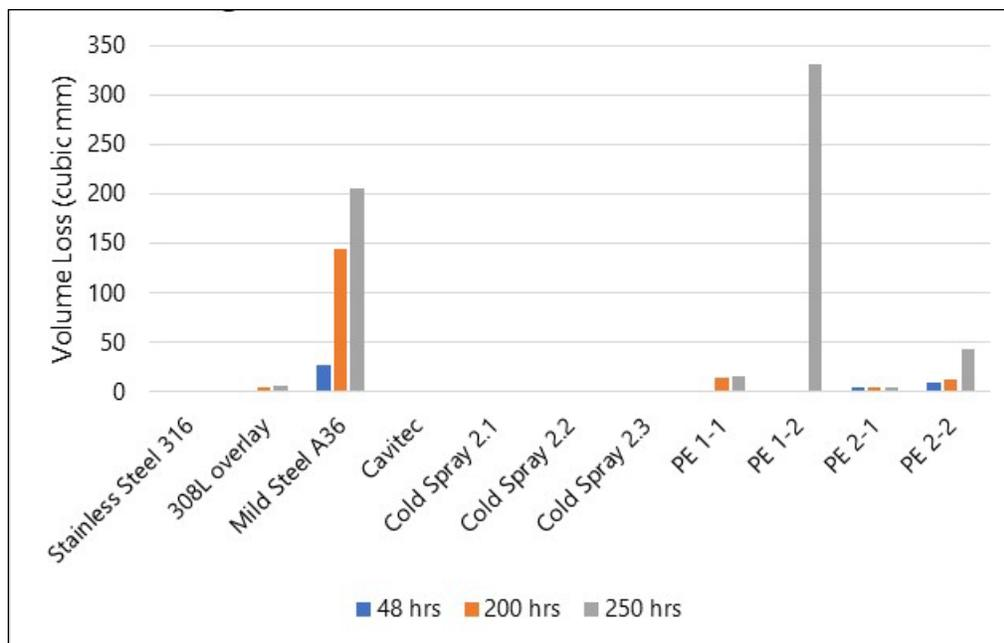
Figure 15.—Long-term testing to evaluate the top performing materials for three test durations reported in hours (hrs).
