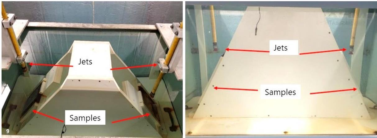
Figure 7.—Top view (left) and side view (right) of submerged jet test set-up.
