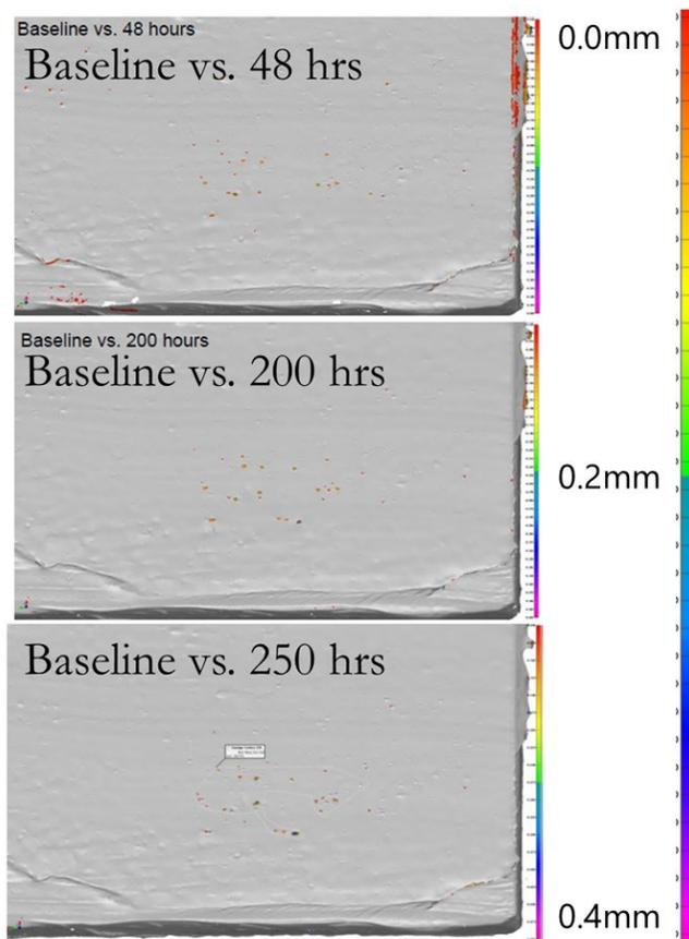
Figure 24.—PE 2-1 long-term cavitation using laser scanner to monitor the microscopic changes. Color bar scale is in millimeters.
