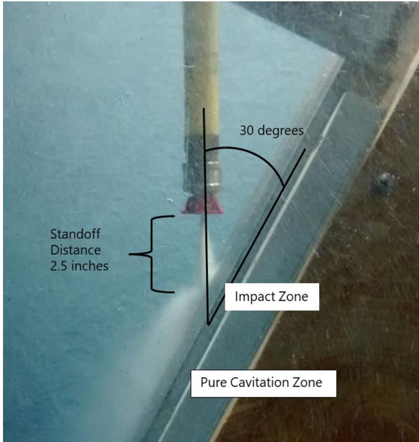
Figure 6.—Image of submerged jet cavitation testing showing the sample angle with the cavitation travelling down the sample, along with the location of the two defining zones of damage.
