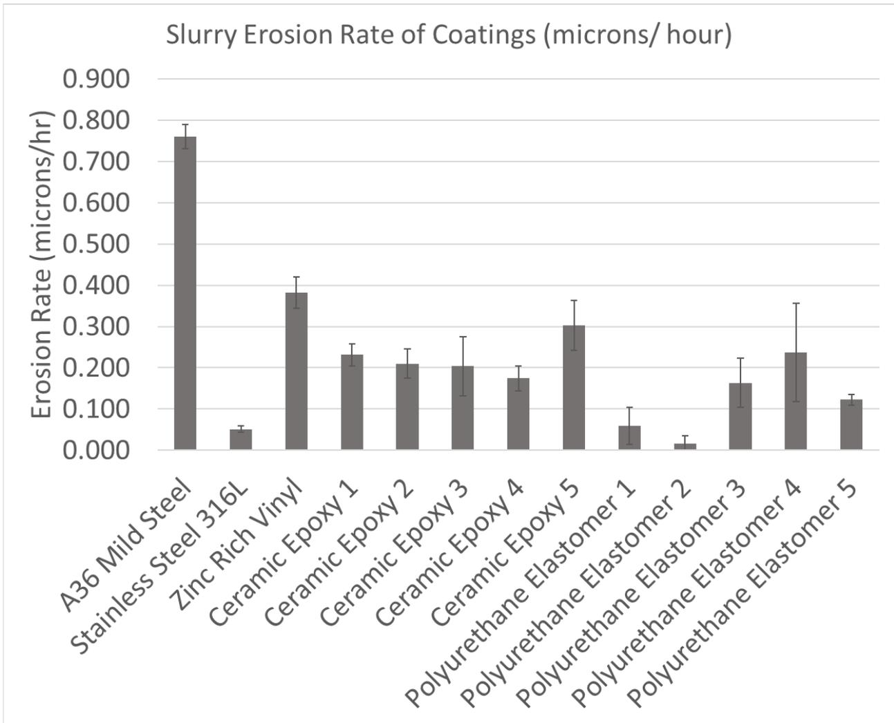
Figure 7. Slurry erosion rate of ceramic epoxy coatings compared to polyurethane elastomers.
