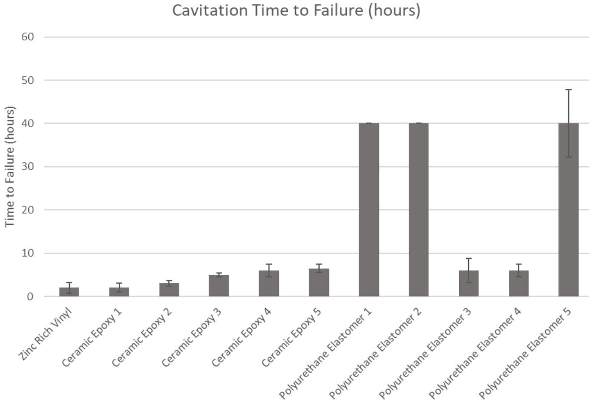
**Figure 6. Cavitation test results for average time to failure to substrate. The ceramic epoxy systems and polyurethane elastomers 3 and 4 failed within six hours of testing compared to polyurethane elastomers 1, 2, and 5, which passed the 40-hour test. Elastomer 5 had some damage but didn't fail to substrate.**
