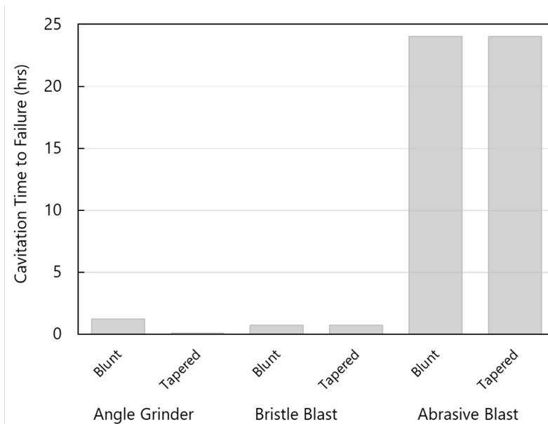
Figure 13.—The effect of different termination details on cavitation time to failure in hours (hrs) for PE 1. Abrasive blast cleaning is necessary to prevent delamination.
