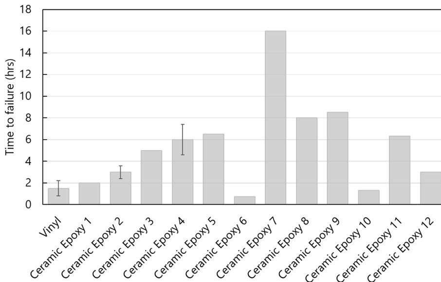
Figure 11.—Cavitation resistance of ceramic-filled epoxy, time to failure in hours (hrs).
