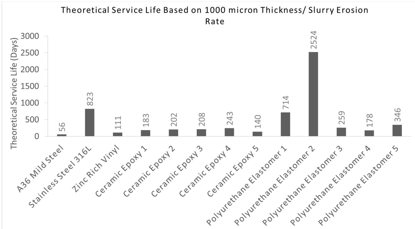
**Figure 8. Theoretical service life for slurry erosion environments.**
