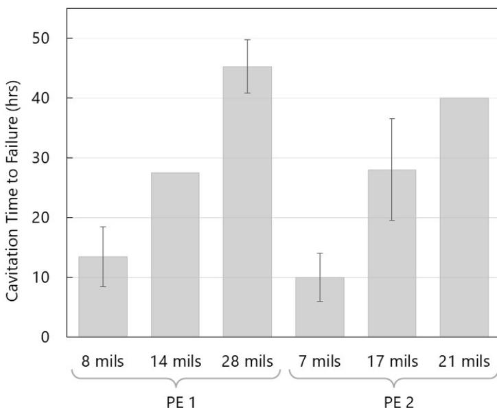
Figure 14.—Elastomer thickness study to determine the minimum elastomer thickness to resist cavitation with time to failure in hours (hrs).
